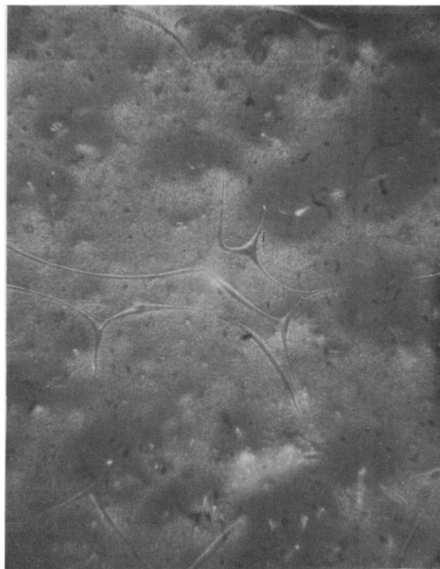
Figure 7 Surface of attached pigmented coating ( \times 67 optical microscope) showing Bénard cells and some pigment agglomeration
